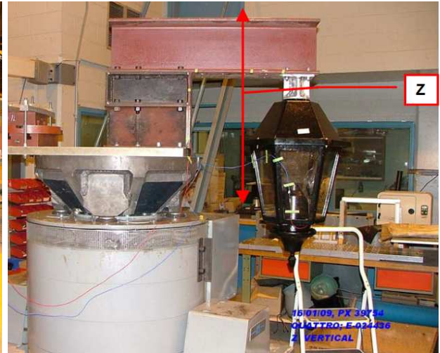
Vibration test on the Vertical Z axis
